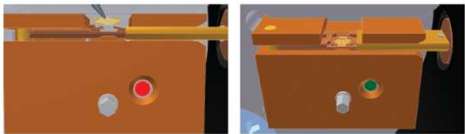
Figure 3. Inserting the specimen grid into the Quickload specimen securing mechanism.
